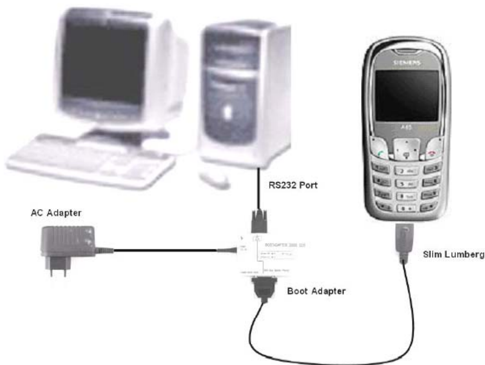
FIGURE 7.1 A65 SERIES SOFTWARE PROGRAMMING SETUP
